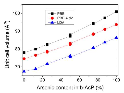
**Supplementary Figure S3** Cell volumes for  $b-As_xP_{1-x}$  calculated with PBE, PBE+d2, and LDA functionals. The PEB and LDA results are from previous studies<sup>[1]</sup> and used as comparisons here.
