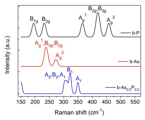
**Supplementary Figure S7** Calculated Raman spectra of black phosphorus (b-P, black), black arsenic (b-As, red), and black arsenic-phosphorus (b- $As_{0.5}P_{0.5}$ , blue, model contains arsenic-phosphorus bonds only). The calculation method is PBE-d2.
