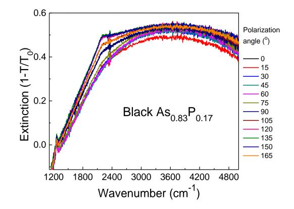
**Supplementary Figure S5** Polarization-resolved infrared absorption spectra of a black- $As_{0.83}P_{0.17}$  flake at different polarization angles of 0 to 165 degrees with a step of 15 degree. Figure 3a in the main text uses part of the spectra (45, 75, 105, and 135 degrees) shown here.
