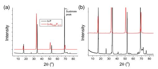
**Supplementary Figure S1** XRD patterns of b-P and b- $As_{0.83}P_{0.17}$  bulk crystals. Plot b is a zoom-in plot of a. The results show that b-AsP has orthorhombic structure, similar to b-P. This result is consistent with our early publication.<sup>[1]</sup> The XRD patterns were collected using a Rigaku Ultima IV powder/thin-film diffractometer with Cu K $\alpha$  line.
