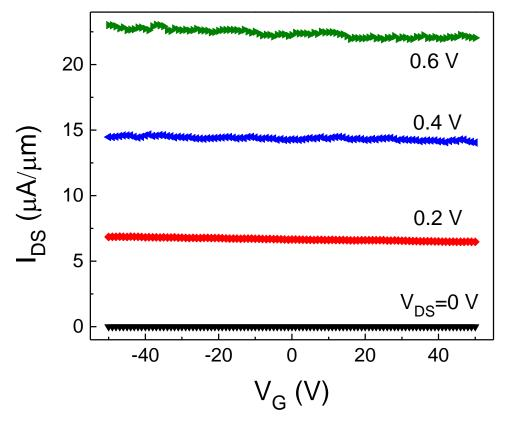
**Supplementary Figure S4**  $I_{DS}$ - $V_G$  characteristics of a representative thick black arsenic-phosphorus flake (b-As<sub>0.83</sub>P<sub>0.17</sub>). The thickness of the flake is around 60 nm based on AFM measurements. The sample is highly conductive and there is nearly no gate dependence for such thick flakes due to screening effect.
