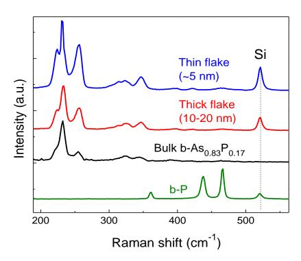
**Supplementary Figure S6** Raman spectra of bulk (black), thick flake (red), and thin flake (blue) of  $b-As_{0.83}P_{0.17}$ . The Raman spectrum of pure b-P (i.e.,  $b-As_0P_1$ ) is also shown as green curve for comparison. The spectra were vertically shifted for clarify.
