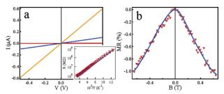
Figure 4. Electrical measurements of individual Fe<sub>3</sub>O<sub>4</sub> nanotubes. (a) I-Vcurves taken at three different temperatures of 290 K (orange), 180 K (blue), and 77 K (red). (Inset) Arrhenius plot (log  $R \approx 1/T$ ) and its linear fitting (blue line). (b) MR measurement at 77 K. Data points are depicted as the red triangles with the blue curve as a guide for the eyes.
