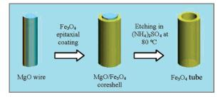
Figure 1. Schematic illustration of the fabrication process of Fe<sub>3</sub>O<sub>4</sub> nanotubes
