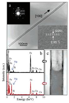
Figure 3. (a) Low-magnification TEM image of an Fe<sub>3</sub>O<sub>4</sub> nanotube, with the SEAD shown in the upper inset. (Lower inset) HRTEM images taken on the tube wall. (b) EDS spectra of solid (black curve) and hollow (red curve) part of a partial ectched Fe<sub>3</sub>O<sub>4</sub> nanotube (c).
