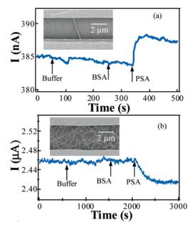
*Figure 3.* Current recorded over time for an individual In<sub>2</sub>O<sub>3</sub> NW device (a) and a SWNT mat device (b) when sequentially exposed to buffer, BSA, and PSA. Insets: SEM images of respective devices.
