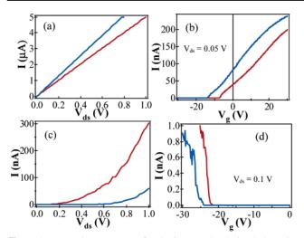
**Figure 2.** I-V and  $I-V_g$  curves of an In<sub>2</sub>O<sub>3</sub> nanowire device (a, b) and a SWNT device (c, d) before and after PSA incubation. Red and blue curves represent measurements performed before and after PSA incubation, respectively.
