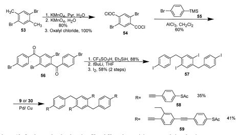
Scheme 12. Syntheses of molecular wires 58 and 59, each containing two methylene barriers.
