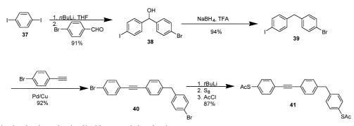
Scheme 7. Synthesis of molecular-scale wire 41 with one methylene barrier.
