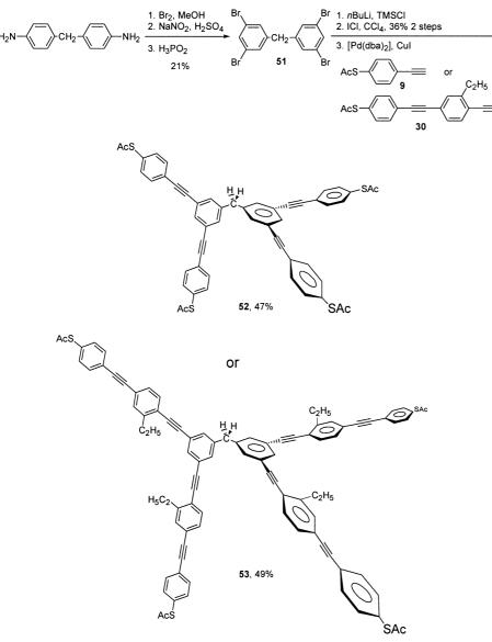
Scheme 11. Syntheses of four-terminal wires 52 and 53, both with one methylene barrier.
