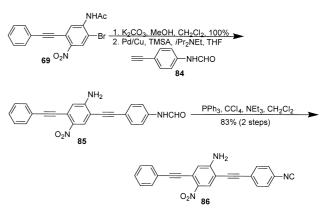
Scheme 20. Synthesis of molecular device  $\mathbf{86}$  with an isonitrile alligator clip.
