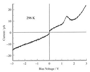
Figure 1. I(V) plot of **48** at 296 K, which shows NDR. The non-symmetric NDR effect may be due to the differences in the self-assembled versus metal-evaporated contacts on either side of the nanopore.
