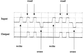
Figure 5. The mDRAM cell input and output that is constructed from **78** in the nanopore. The mDRAM was built into a circuit that had a transistor and a comparator (as do most commercial solid state DRAMs) and operation was at 300 K.
