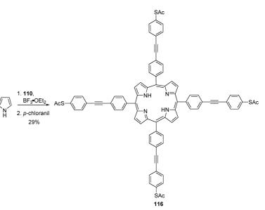
Scheme 26. Synthesis of four-terminal porphyrin 116.
