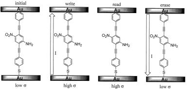
Figure 4. Write, read, and erase sequences for **70** in the nanopore and its use as a one-bit random access memory.
