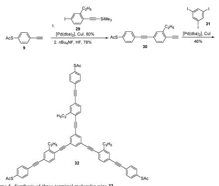
Scheme 5. Synthesis of three-terminal molecular wire 32.
