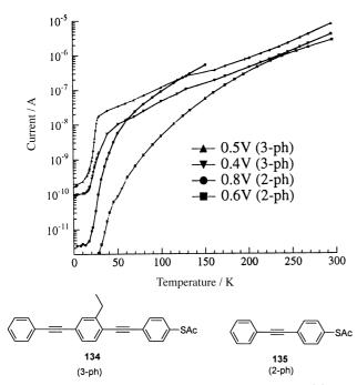
Figure 2. Plot of current versus temperature of compounds **134**<sup>[20]</sup> (3-ph) and **135**<sup>[43]</sup> (2-ph) in the nanopore with a bottom contact (SAM-contact side) of gold and a top contact of titanium. Each nanopore contains approximately 1000 molecules.
