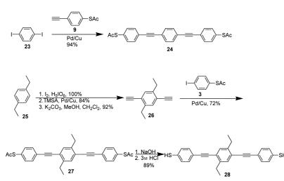
Scheme 4. Syntheses of two-terminal molecular wires 24 and 28.
