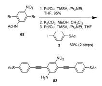
Scheme 19. Synthesis of two-terminal molecular device 83.
