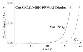
Figure 9. Copper (SAM)/MEH-PPV/Al diodes demonstrating improvement of charge injection from Cu using the NO<sub>2</sub> terminated SAM, **136**. The current in the devices is dominated by hole injection from the Cu contact (the Al electrode is a poor electron injector) so the increased current from the Cu/SAM electrode (compared to the Cu electrode that does not bear a SAM) indicates improved injection from that contact. The MEH-PPV film thickness is 100 nm in both cases.
