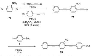
Scheme 17. Synthesis of mononitro molecular device 78.
