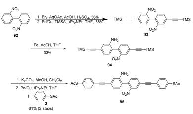
Scheme 22. Synthesis of nitro-amine biphenyl compound 95.
