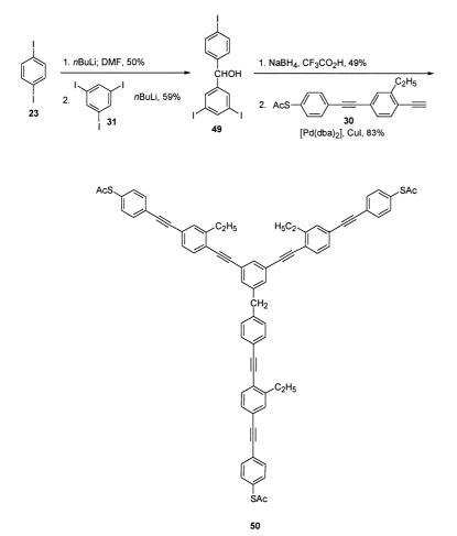
Scheme 10. Synthesis of three-terminal molecular wire 50 with one methylene barrier.
