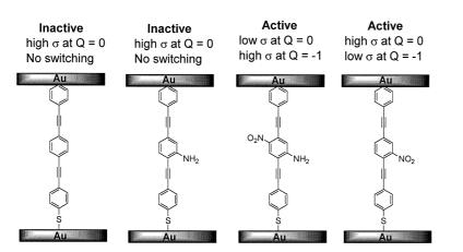
Figure 6. Summary of the mNDR and mDRAM results obtained to date in the nanopore cell where  $\sigma$  is the conductance and Q is charge. "Inactive" and "Active" refer to the device properties wherein a large nonlinearity in the I(V) curve results upon application of a voltage.
