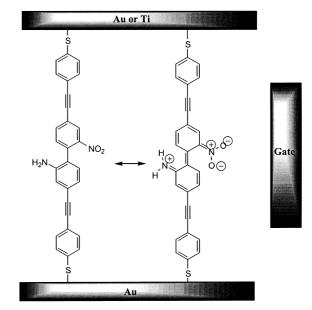
Figure 7. Schematic of a molecular device controller where a gate electrode could modulate the overlap in a molecule by preferring the more planar zwitterionic form.
