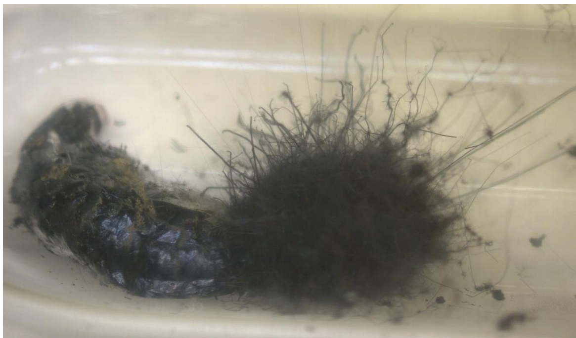
Figure S6. An optical image of P_{20.56(1)}Sb_{0.44(1)} located inside an ampoule after synthesis. On the left-hand side the bulky residue is a lead regulus, while on the right hand side are bundles of fine needle-shaped P_{20.56(1)}Sb_{0.44(1)} .
