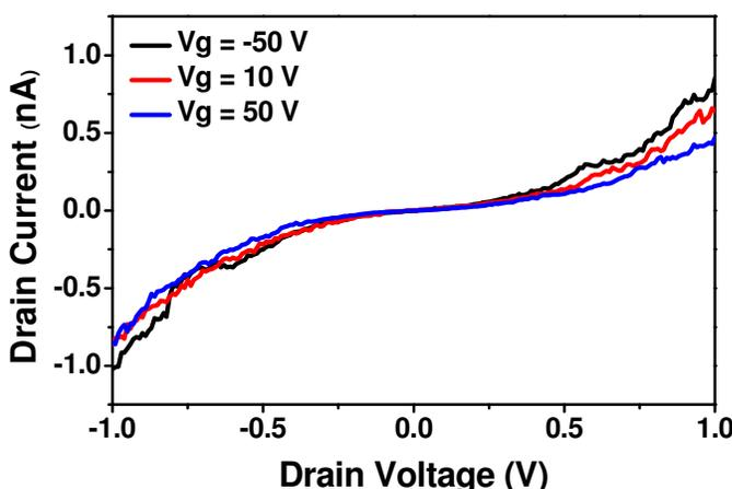
Figure s5.  $I-V_d$  curves of an individual GNR device at different gate biases. The weak P-type gate modulation is attributed to the electric field screening effect by the closely positioned source-drain.
