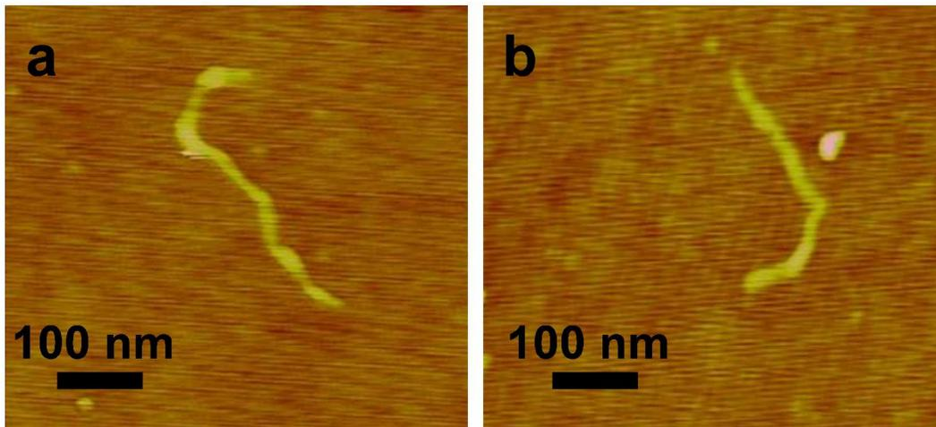
Figure s2. AFM images of typical individual GNRs on dodecyltriethoxysilane functionalized  $\text{SiO}_2$  surface showing lengths of 300 to 500 nm.
