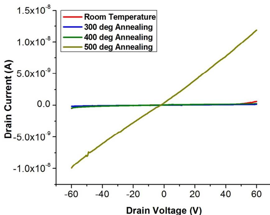
Figure s6. I-V<sub>d</sub> curves of a device before annealing, and after annealing at 300 °C, 400 °C, and 500 °C showing significant enhancement in conduction after annealing at 500 °C.
