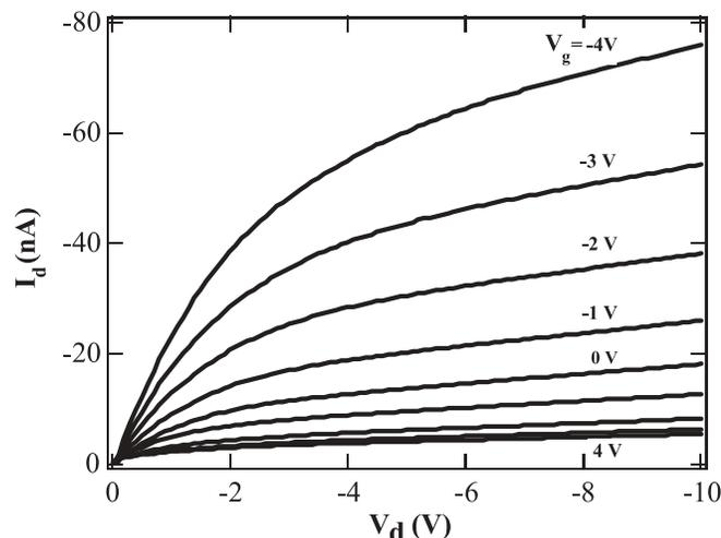
**FIGURE 2**  $I_d - V_d$  characteristics of the polymer transistor exhibiting low operation voltages. The gate bias varies from  $-4\text{ V}$  to  $+4\text{ V}$  with 1-V increment from the top curve to the bottom curve. The channel width is 500  $\mu\text{m}$  and the channel length is 2  $\mu\text{m}$  for this device
