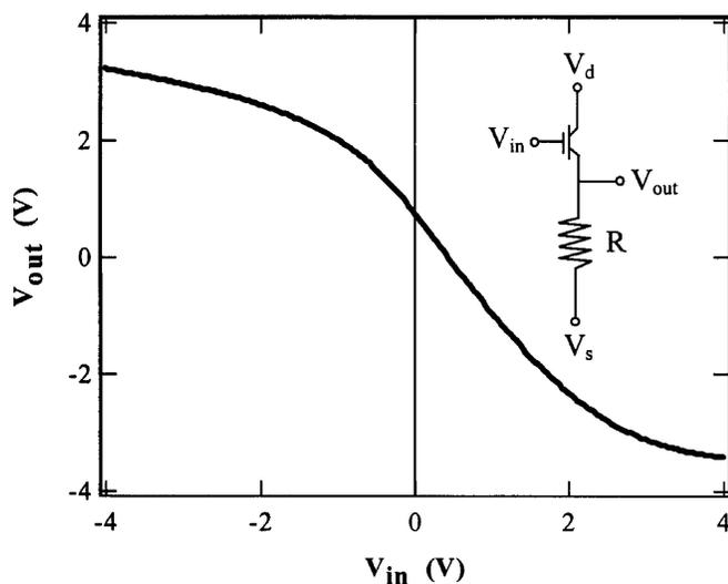
**FIGURE 4** Input-output characteristics of the polymer-based inverter with the circuit diagram shown in the inset
