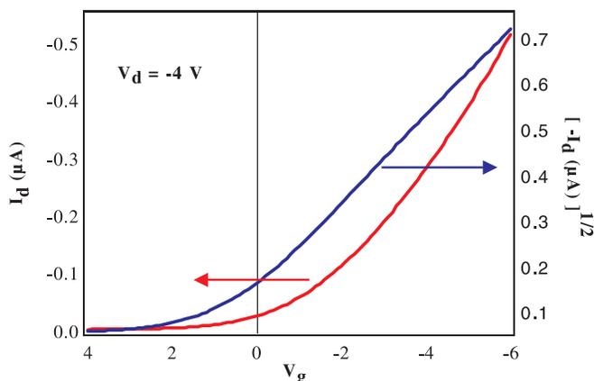
**FIGURE 3** Transfer characteristics of the polymer transistor:  $I_d - V_g$  shown as the red line and  $(-I_d)^{1/2} - V_g$  shown as the blue line. The threshold voltage and the mobility can be derived
