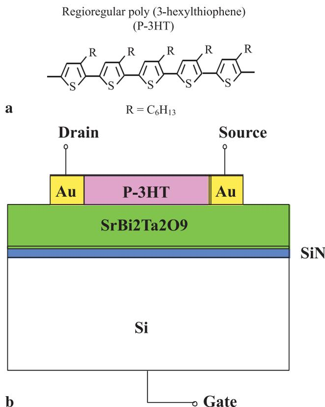
**FIGURE 1** **a** Formula of regio-regular poly(3-hexylthiophene) (P-3HT). **b** Schematic diagram of the polymer field-effect transistor with high-dielectric SBT film as the gate dielectric
