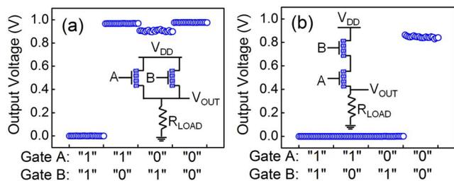
FIG. 4. (Color online) Output characteristics of (a) NAND and (b) NOR, with resistive load. Inset: schematic of the circuits. The supply voltage for both circuits is  $V_{DD}=1$  V. Input voltages of 2 and  $-2$  V are treated as logics 1 and 0, respectively.
