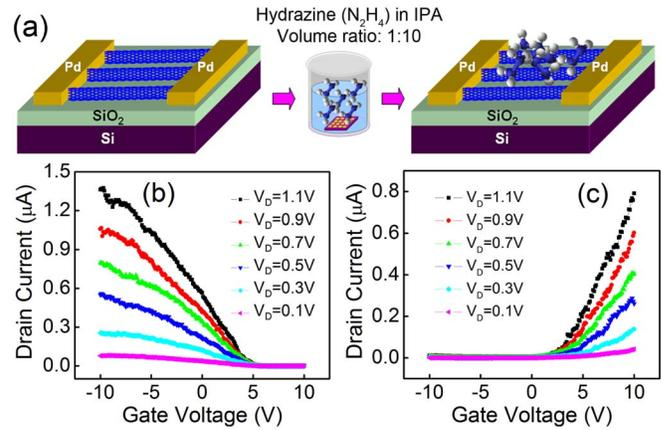
FIG. 2. (Color online) (a) Schematic drawing depicting the hydrazine doping process. (b)  $I_D$ - $V_G$  curves of the device before hydrazine doping. (c)  $I_D$ - $V_G$  curves of the device after hydrazine doping.
