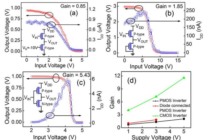
FIG. 3. (Color online) Voltage transfer characteristic (red curve) and power supply current (blue curve) of (a) the PMOS inverter, (b) the diode-loaded inverter, and (c) the CMOS inverter. Inset: schematic of the circuits. The supply voltage is  $V_{\text{DD}}=1$  V for (a) and (c), and  $V_{\text{DD}}=3$  V for (b). (d) Curves showing the dependence between the gain and supply voltage of different types of inverters.
